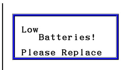
If you try to continue using the calculator, it will automatically turn off in order to protect memory contents. You will not be able to turn power back on until you replace batteries.
