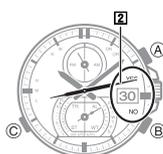
In the Timekeeping Mode, press **B**. The **2 Second Hand** will move to **H (High)**, **M (Mid)**, or **L (Low)** to indicate the power level, and then it will indicate the latest time calibration signal receive operation result.
