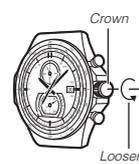
The crown of this watch is a screw in lock crown. Before using the crown, you must first rotate it towards you to loosen it.
