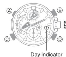
13. Rotate the crown to align "1" in the center of the day indicator.
