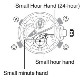
9. Rotate the crown to align the small hour hand, small minute hand, and small 24-hour hand with 12 o'clock.
